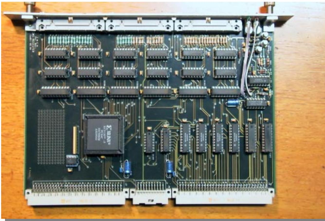
**A 48 input channels VME I/O register accepting TTL differential signal levels for data acquisition system.**
