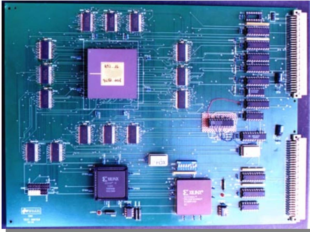
**A VME Test Board to verify the performances of the SORTER processor developed in  $0.8 \mu$  BiCMOS technology and developed for the muon trigger system of the CMS experiment. The board contains some FIFO's to test the internal Boundary Scan structure of the SORTER. It runs with a 66 MHz as a maximum master clock, to test completely the SORTER performance.**
