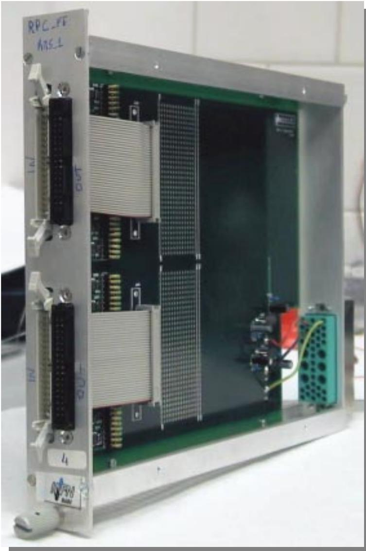
**An LVDS Receiver module, has been built to receive LVDS digital signals and convert them into ECL output signals. This NIM module contains a total of 32 channels and it has been designed to convert the Low Voltage Differential Signals used to achieve high data rate, low power and to reduce EMI effects in signals transmission, into ECL signals, used in standard data acquisition modules.**
