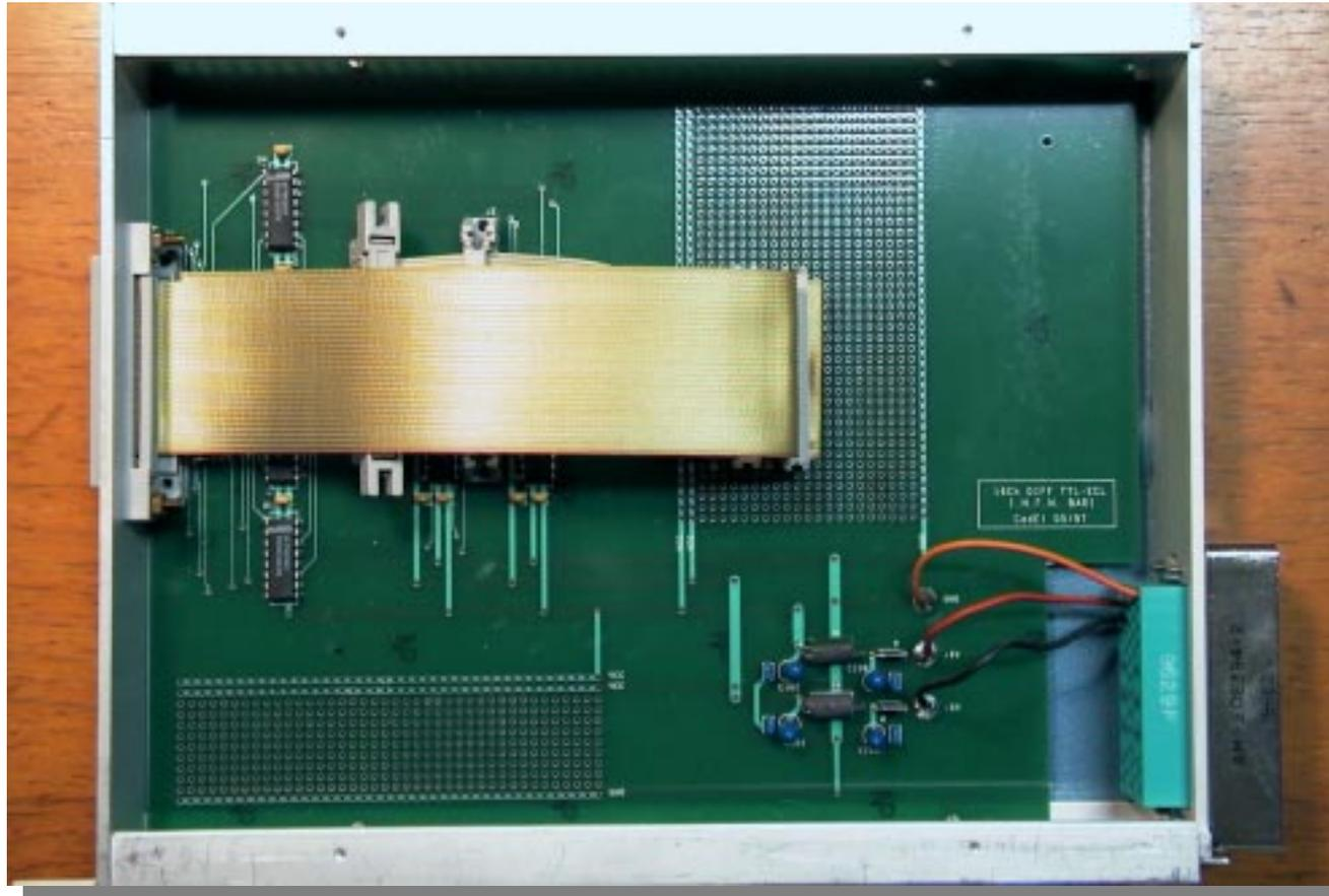
**A 16 Channels Differential TTL\_ECL Converter useful to receive differential pairs signal and to convert in ECL to input in standard NIM/CAMAC/VME modules**
