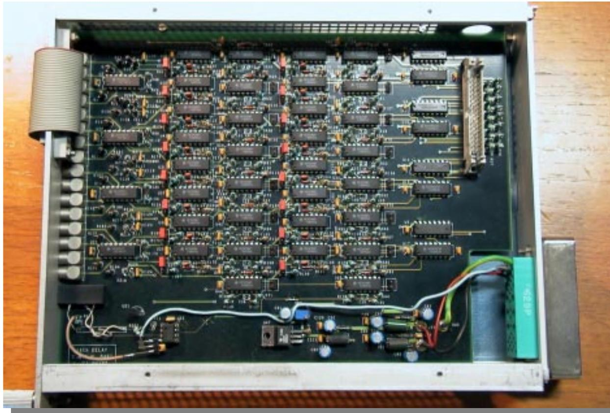
**A 16 channels TTL- NIM converter used to receive TTL differential signals and to convert them into NIM output signals, with the possibility to set a programmable delay (0-200 ns) on output, useful for triggering purposes.**
